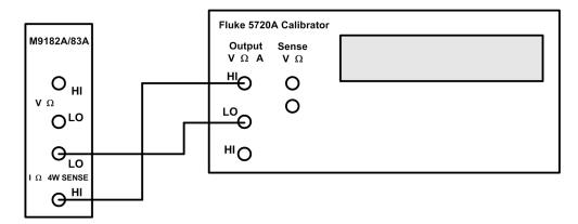
2 Apply the input signal shown in the "Input" column of the table. Enter the actual applied rms input voltage (see "Adjustments" on page 27).
