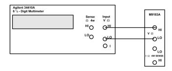
4 Program each output voltage on the M9182A/83A DMM in the order shown below. Measure this voltage with the external DMM. Compare these measurement results to the appropriate test limits shown in the table. Be certain to allow for appropriate source settling.
