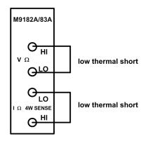
2 Now Perform the calibration process (see "Calibration Process" on page 25). Enter the calibration value of 0.00 for the calibration value (because the source is 0 V).
