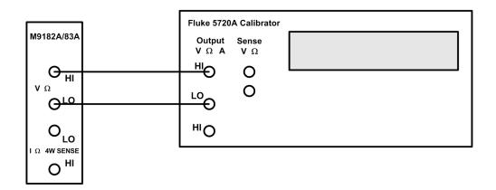
2 Apply the input signal shown in the "Input" column of the table. Enter the actual applied input voltage (for AC voltages enter RMS value) (see "Adjustments" on page 27).
